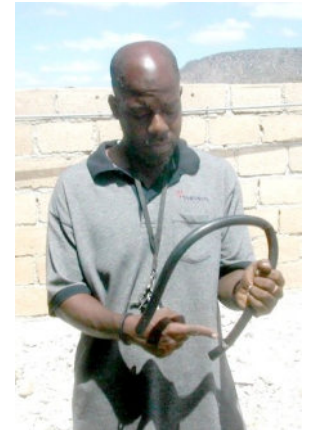
Brooklyn John pointing to the kink we cut out of the line we replaced.
