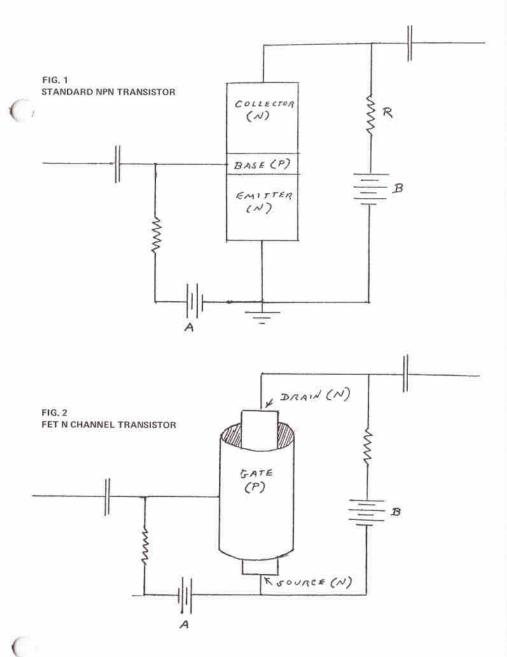
In this case, C is a piece of silicon with an excess of electrons doped into it. So it is "N" meaning negative. Welded to it is B, a very thin sheet of
