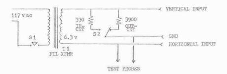
The unit to be checked is connected across the test leads and S1 activated. For diodes and transistors, a solid horizontal bar = open; solid vertical bar = short. Proper conduction will show as a sharp right angle.
