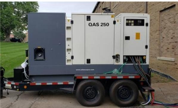
powerful RF super quiet generator on a trailer. The generator was big enough to generate enough power for two buildings and the field-house!! They provide a 120 amp panel with approximately 60 outlets.
