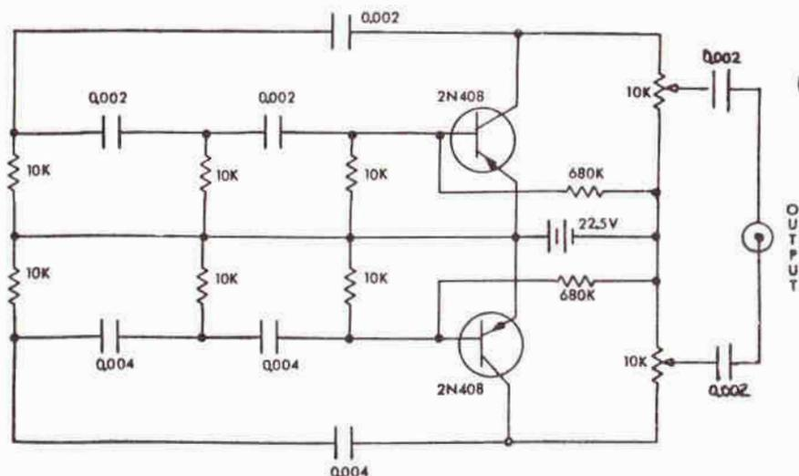
Sooner or later in the course of adjusting a single sideband transmitter you are going to need a two-tone signal. There are many ways of obtaining two audio signals for such adjustments; however, here is a simple solid state circuit that can be built in a small minibox. Power levels in the circuit are low, so  $\frac{1}{4}$  watt resistors can be used. The potentiometers can be of the small variety and the capacitors can have voltage ratings as low as 25 volts.
