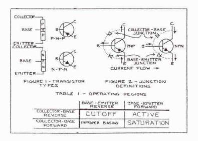
Figure 2 shows the junction definitions and imaginary back-to-back diodes are sketched to represent them. Normal direction of current flow is also given. NOTICE THAT THE ARROW IN TRANSISTOR THE SYMBOL POINTS IN THE DIREC-TION OF NORMAL. EMITTER CURRENT FLOW (assuming current from positive to negative).
