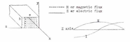
The electric force is along the y axis just as if the top and the bottom of the guide were the two plates of a condenser, only the stress dies to zero at the edge of the guide along the z axis. The magnetic lines of force are closed loops and look like whirlpools inside the tube. In order to have our electric and magnetic ines of force in the positions shown above, the radiating element must be perpendicular to the z axis.
