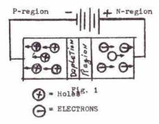
WHY, with reverse bias, there is no conduction by majority carriers. Fig. 1 shows that the holes in the P-region and the free electrons in the N-region move away from the junction under the attraction of the opposite charges provided by the battery. The result is to greatly widen the depletion region.
