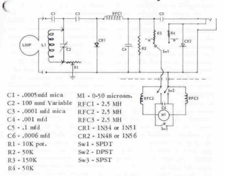
Build a better mousetrap and the world will beat a path to your door. This gadget about to be described is not a better "mousetrap" so to speak, it's not a new idea, it has probably been built or constructed many times before. Circuits such as this have been in existence since the invention of the crystal. However, this instrument
