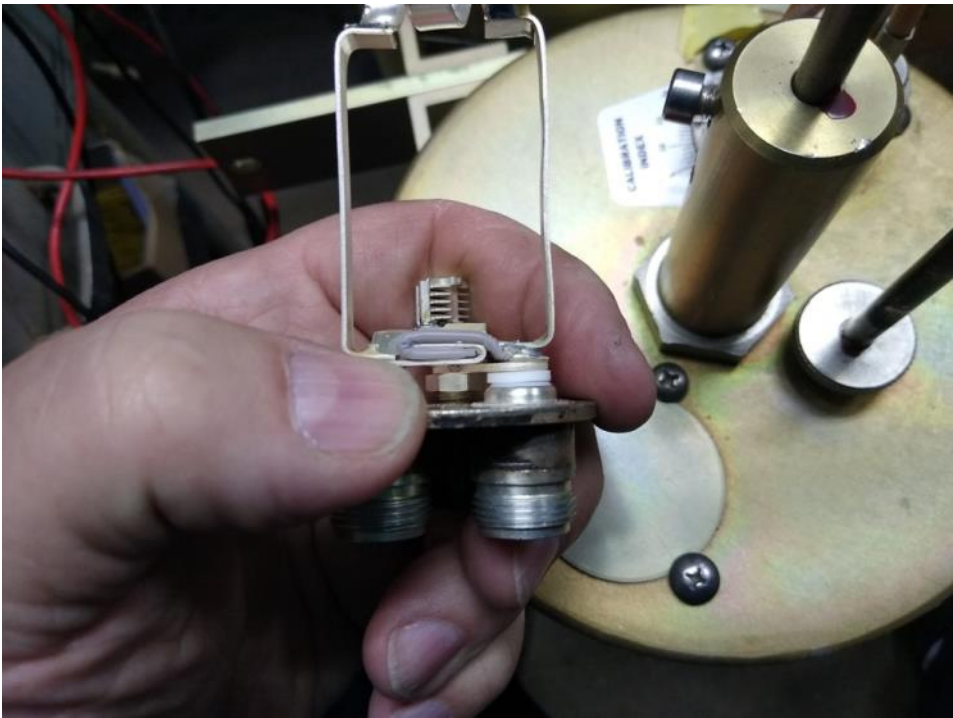
Photo 'E' - This photo shows the insertion loop with the Z-shaped capacitor almost touching the strap. ..No space between them can be seen. The small trimming capacitor behind it is the notch adjustment.
