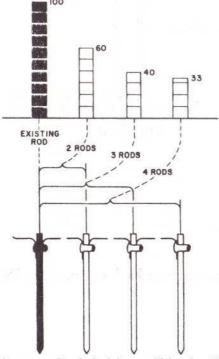
Average results obtained from multiple-rod earth electrodes.
