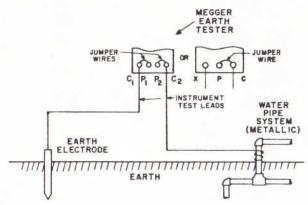
Two-Terminal earth-resistance test.
