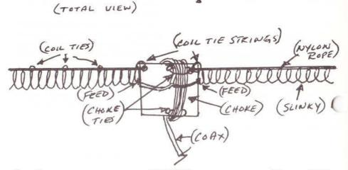
slinkies don't slip or move around, take a needle with some heavy thread and about every 5 or 10 coil loops poke the needle through the rope and tie it around the loop. This should keep the coils uniform. The antenna is not signed to be resonant on 160 without a tuner, so one is needed. It is easy to load up and a fantastic radiator for its size. The antenna tends to radiate a little better the longer it's stretched out.
