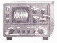
The SM-220 is an extremely useful and unique station monitor. It allows you to monitor your transmissions, monitor incoming signals and monitor the amount and strength of band activity and performs as a general purpose 10 MHz oscilloscope, as well.
