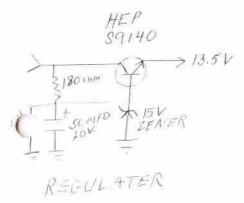
Another advantage it gives you is filtering. Besides being called regulators, these circuits are also called electronic filters, capacitance multipliers, etc. So, besides the advantage of regulation you also get additional effective filtering.
