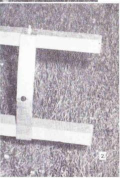
it consists of a piece of metal bent to allow the 2 x 4's to come up along side of the pole. Slots should be cut in strap to allow adjusting the tilt section to exact vertical. A hole was drilled in the pole and the strap and a long bolt run all the way through the pole to securely lock the tilt section.
