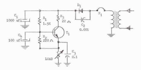
The signals fed into the transistor T1 collector are half wave rectified DC pulses. The output signal taken from the emitter is a filtered regulated DC voltage. The AC supply is half wave rectified by D1 and filtered by C1; F1 is a fuse normally formed by a chemical composition designed to protect transistor T1 in event of a short developing on the load side of the transistor. C2 is a radiation preventive measure placed across the half-wave rectifier whose value is normally .001 micro-farad.
