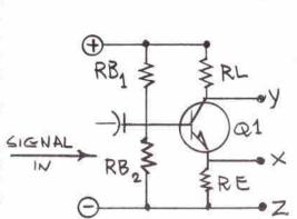
If RE and RL are made the same resistance value, the signal between Y and Z and Z and X will be the same peak to peak value but 180 degrees out of phase with each other. We thus have a typical phase inverter circuit used to feed a push/pull output stage.
