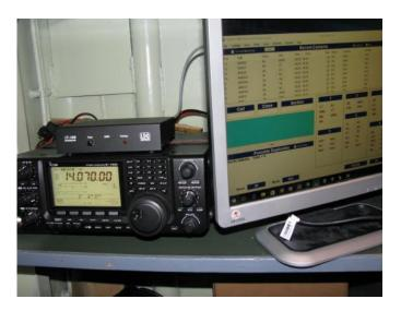
Inside the Ships Radio Room. Although this one was setup for SSB on the 20 Meter Band, They also had Digital on 15, 20 and 40 Meters.
