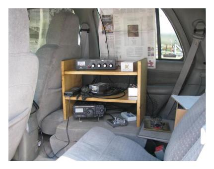
This is Fred's KBOLF CW Station setup in the back seat of his SUV. Note he can use either a Bencher Paddle or a Straight key.
